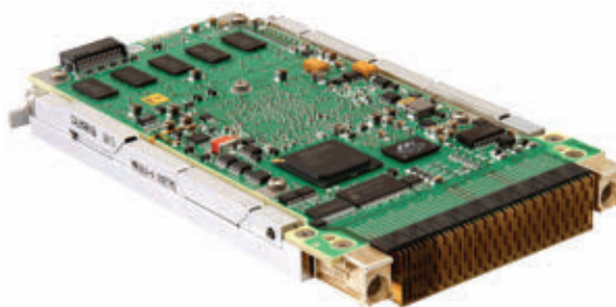
The VPX-150 is a COTS board manufactured by Curtiss-Wright to meet DO-254 and DO-178 safety-certifiable requirements.
